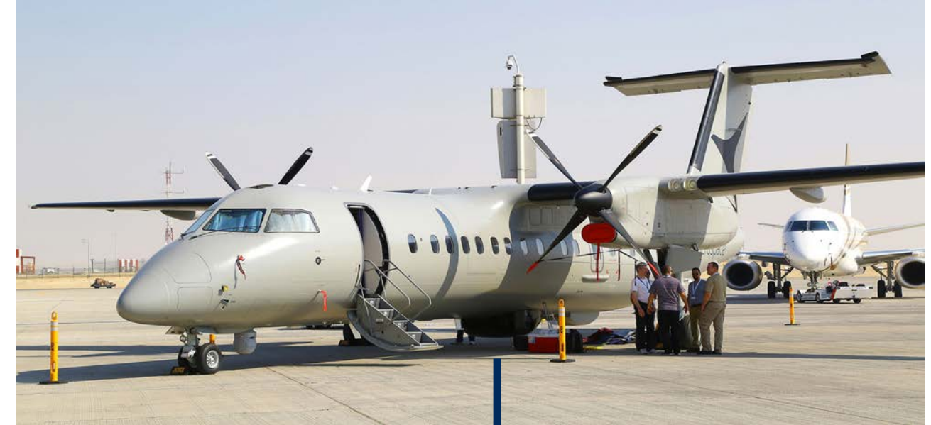
A NUMBER OF THIRD-PARTY AEROSPACE COMPANIES OFFER CONVERSION OF EXISTING CIVILIAN PLATFORMS SUCH AS THIS EXAMPLE OF A DASH 8 Q300 COMMUTER – FITTED WITH SEARCH RADAR, EO/IR, SATCOM AND DISPENSING SYSTEM. THE DASH 8 Q300 REPRESENTS A CREDIBLE MARITIME SURVEILLANCE MACHINE.
