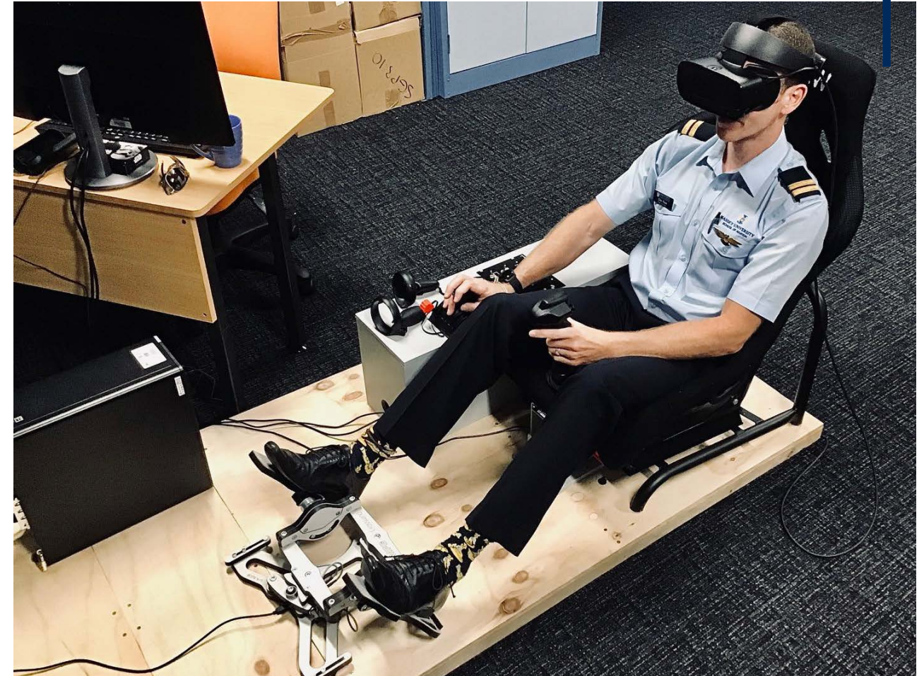
A MASSEY AVIATION SCHOOL FLIGHT INSTRUCTOR CONDUCTS TESTING ON A PROTOTYPE VR FLIGHT TRAINING DEVICE.
