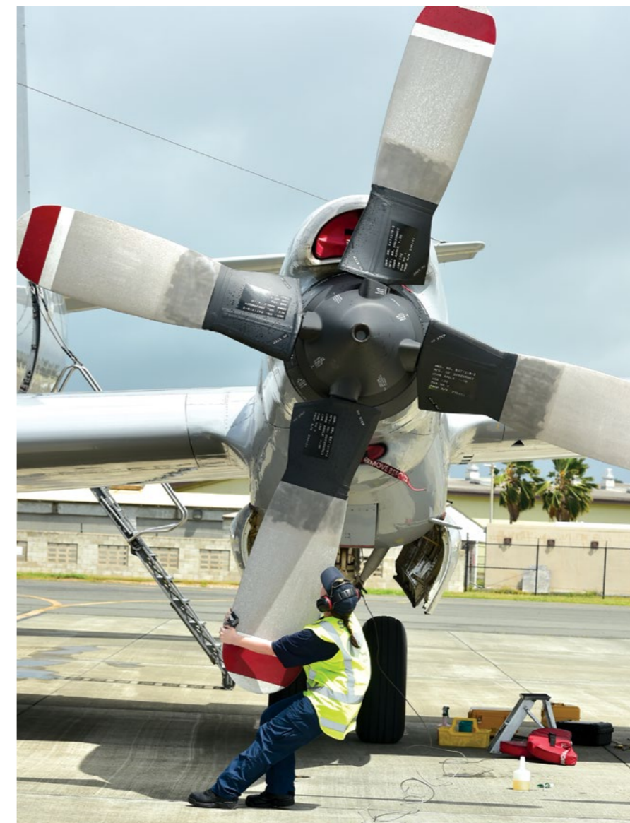
An RNZAF aircraft technician inspecting propeller blades for damage after a mission NZDF Official
